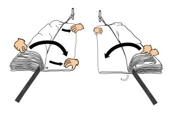
**6.** Be certain to have an equal panel ( gore) count on each side ( the panel numbers may vary with other parachute models ). Be precise and verify that the bottom of the skirt ( leading edge ) is perfectly aligned and tidied..
