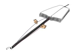
**9.** S-fold the left side of the canopy under the centre of the parachute, then S-fold the right side of the canopy onto the centre of the chute. Keep the canopy neatly folded in place using sandbags or books.
